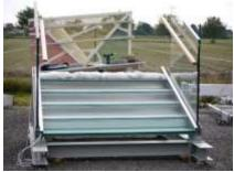
Figure 1. The stair mock-up with specimens installed: "Step 8.15.15.8" (lowest one), "Step 8hs.12hs.12hs.8hs" (other steps) and "Barrier 12t.12t" (barrier glazing).
