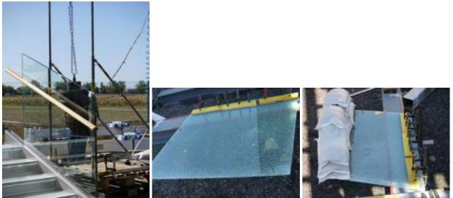
Figure 7. Tests of "Barrier 12t.12t" specimens for soft body impact and linear distributed load.
