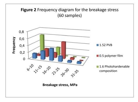
In the obtained results we can see relation between variation coefficient of the ultimate strength and the laminating film type and thickness. Variation coefficient is lower for the modern films even with lesser thicknesses comparing to PVB-film.
