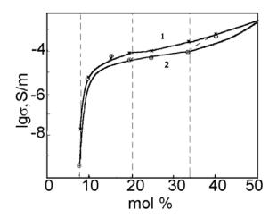
Fig. 2. Electrical conductivity of  $Li_2O$ -SiO<sub>2</sub> glasses after different heat treatment at t=150°C [2]:1 - hardened; 2 - the annealed.
